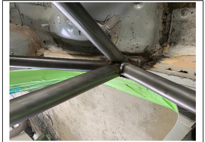
PHOTO 4 MAIN ROLLBAR TO FLOOR ATTACHMENT
