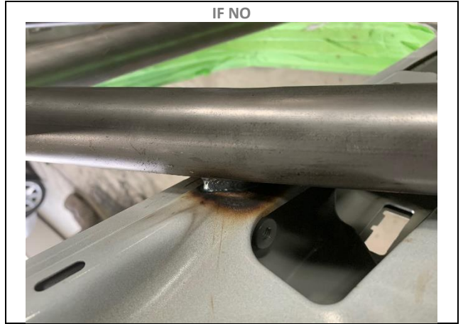
PHOTO 8 MAIN ROLLBAR TO "B" PILLAR ATTACHMENT
